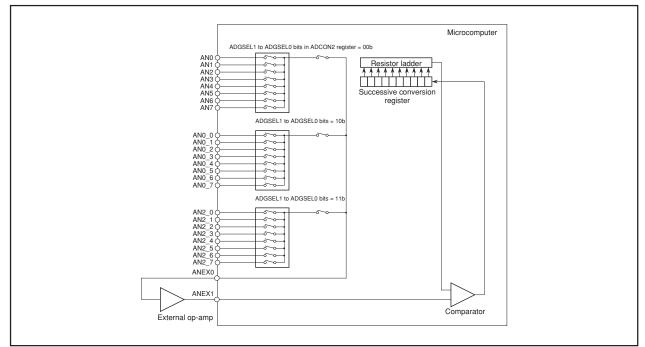
Figure 15.9 External Op-Amp Connection
